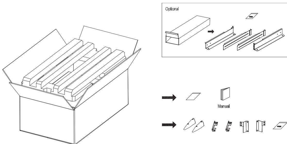
**Figure 3-2: Unpacking the carton of 10K UPS**
