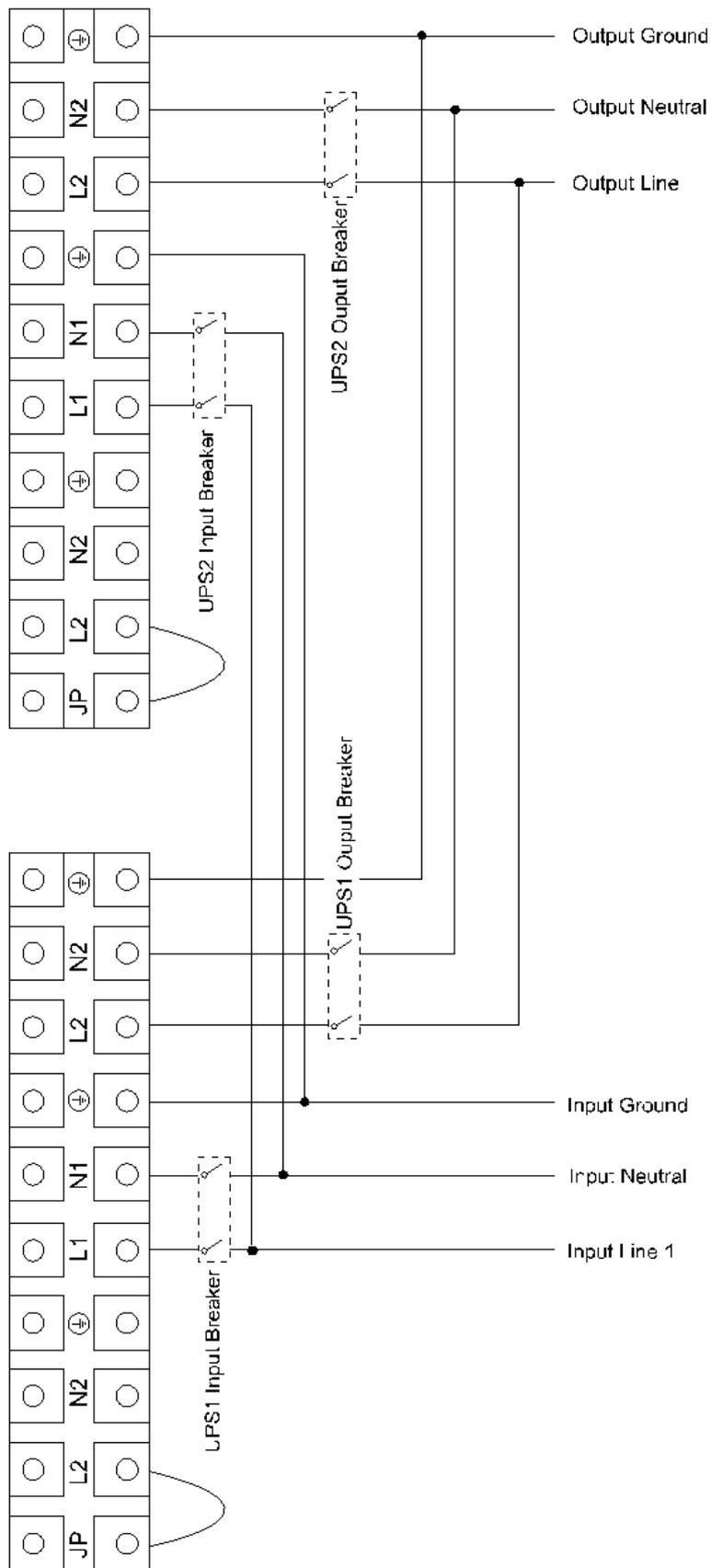
Figure 4-5.a: Parallel system wiring diagram of 6K/10K
