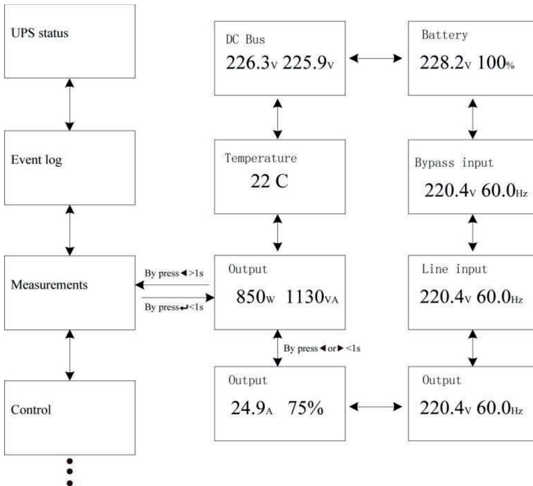
Figure. 5-16 Measurement menu tree
