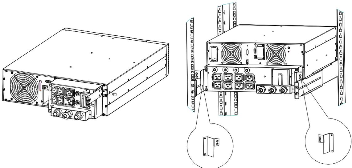
**Figure 3-12. Install the PDU's ears to the UPS**
