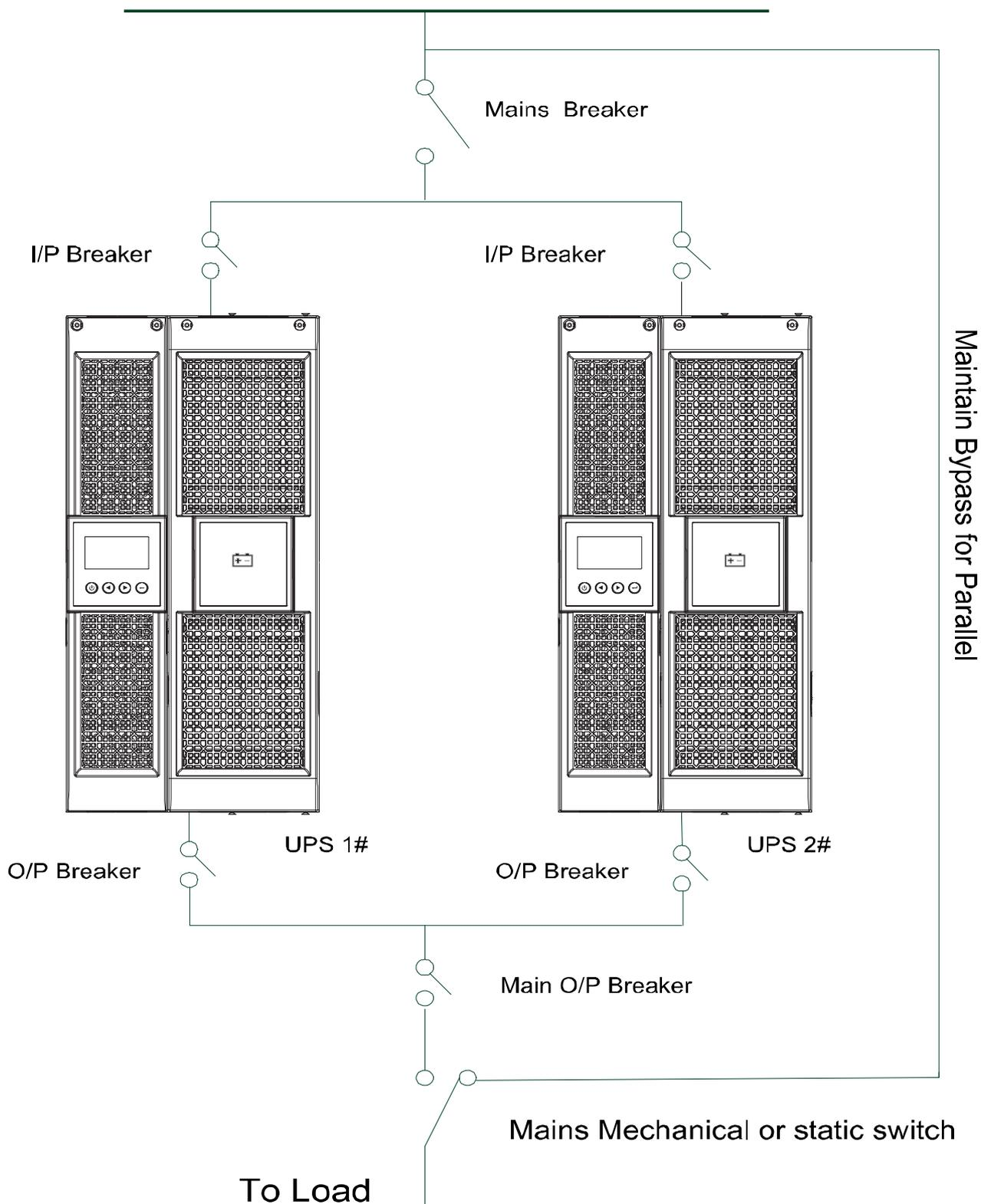
Figure 4-5.b: Parallel System Installation Diagram
