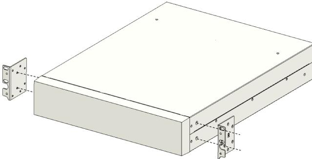
3. Slide the unit into 'rail kit' and make sure tighten the 'rack mounting screw'.
