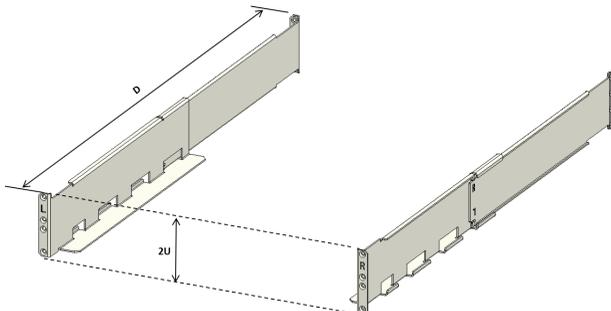
Fasten the rail kit to the cabinet with 8pcs M5 screws + washers (as below):
