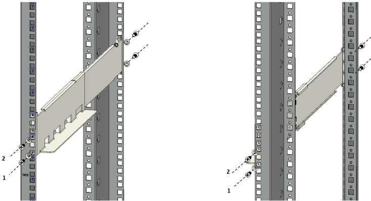
2. Install 'Rack ear' to the unit by the M4 screws(flat head).
