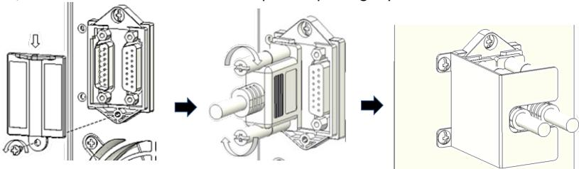
It is recommended to lock the 'parallel cable' (as above) for preventing the parallel ports suffering an unexpected pulling-force and causing the parallel system fault.
