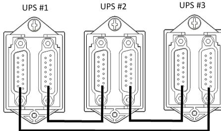
Remove the cover of 'parallel box', then connect each UPS one by one with 'parallel cable', make sure the cable is screwed to parallel port tightly.
